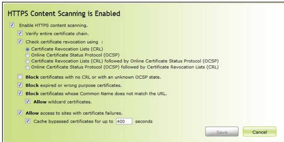
Figure 3: Enabling HTTP decryption: Policy Center > Global Web Policy > HTTPS Content Scanning.
